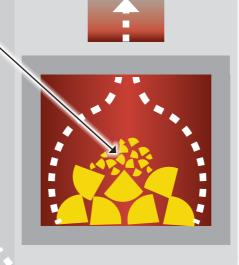
**Adjust the airflow** from below the grate and with the hatches.
